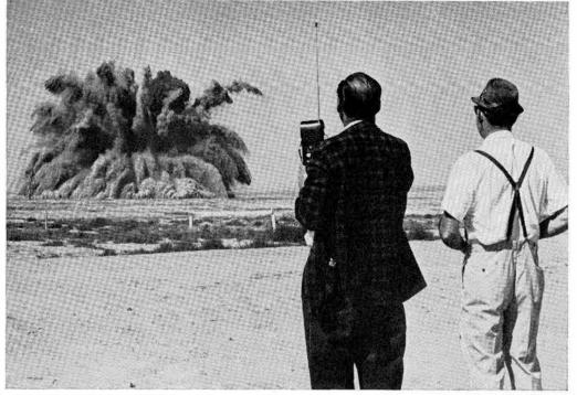
DETONATION of a buried charge of 30,500 pounds of conventional high explosives in Coyote Canyon Test Field created a dust cloud and a crater about 30 feet deep and 105 feet in diameter. The blast was part of a Plowshare experiment to study air-blast geometry. At left is Virgil Harris (9133), Field Test project engineer, with L. J. Vortman (7111), scientific advisor for the project.
